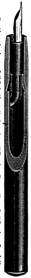
Sectional view of "Jointless," showing "Lucky Curve" and "Spring Lock" in position in barrel.
